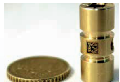
High contrast marking on highly reflective metal
